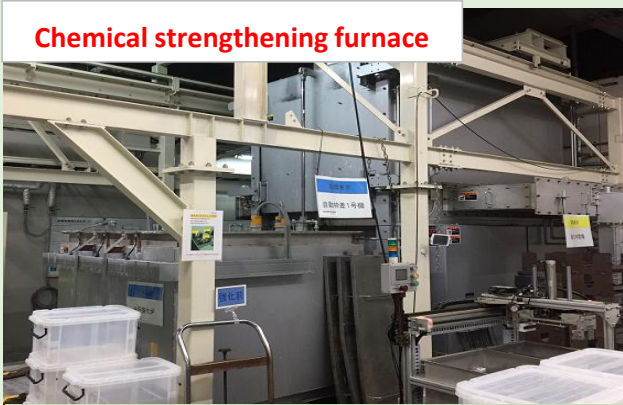
Temperature condition is controlled under strain point (400°C-450°C) for customers' requirement specifications to make Na + transfer into K + .
