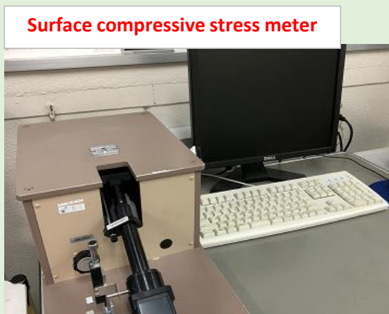
K + ion is bigger than Na + ion, so that compression layer will be constructed around the glass surface, then the glass is stronger not to be broken easily.
